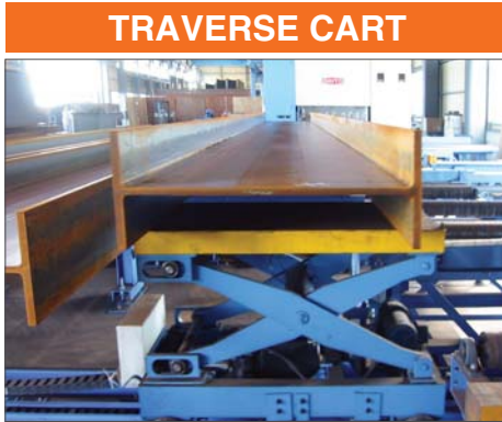
The workpiece is lifted and carried to multiple positions.
