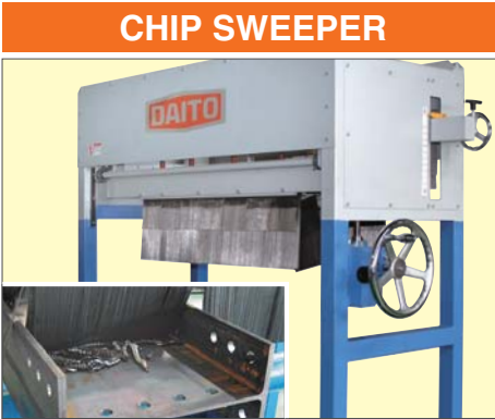
Built-up drill chips are swept away during the workpiece feed.
