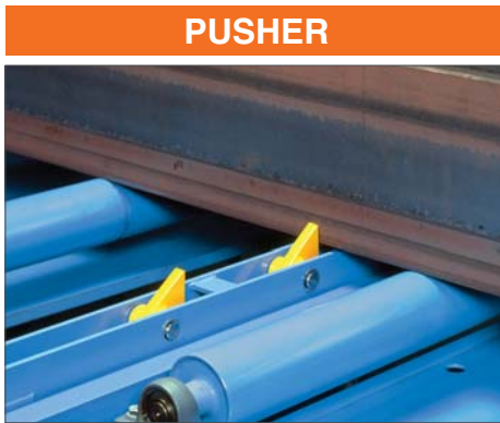
The workpiece is pushed against vertical rollers for precise alignment.
